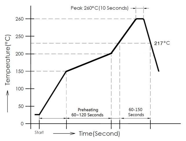
This profile is the minimum requirement for evaluating soldering heat resistance of components. Heat transfer method used for reflow soldering is hot air convection. The actual air temperatures used to achieve the specified profile largely dependent on the reflow equipment.
